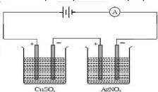
(iii)Applying Faraday's 2nd law of electrolysis, Weight of copper deposited(W1)  $\alpha$  Equivalent weight of copper (E1) .....
